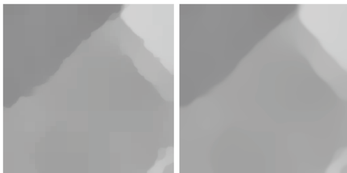
Figure 10: Left: the image filtered by the Perona–Malik filter. Right: Applying of the mean curvature flow filter.
