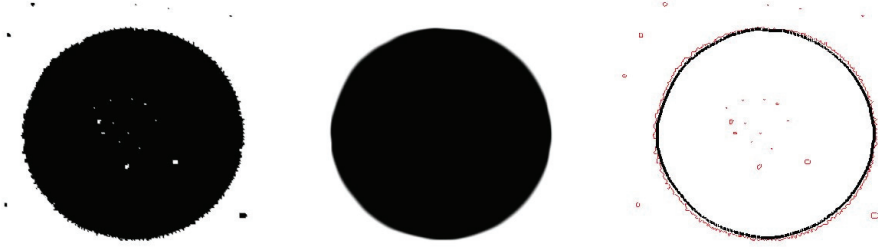
Figure 7: MCF filter smooths the boundaries and removes noise with a high curvature.
